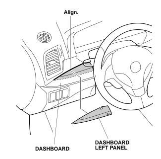
8. While applying light pressure against the dashboard left panel, carefully remove the adhesive backings.
