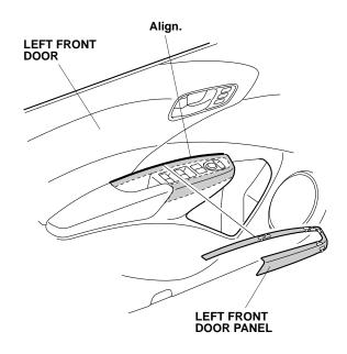
4. While applying light pressure against the left front door panel, carefully remove the adhesive backings.
