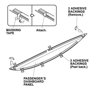
25. Align the passenger's dashboard panel and attach it as shown.
