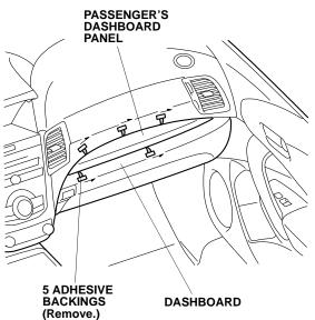
27. Using your hand, firmly press the passenger's dashboard panel against the dashboard.
