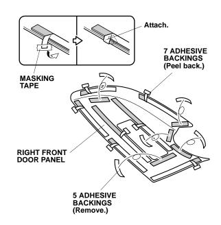
21. Align the right front door panel and attach it as shown.
