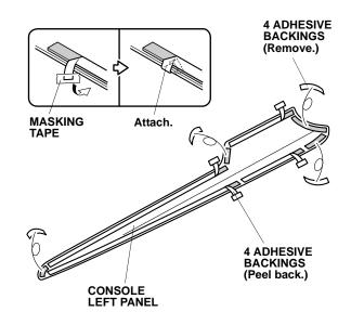
15. Align the console left panel and attach it as shown.
