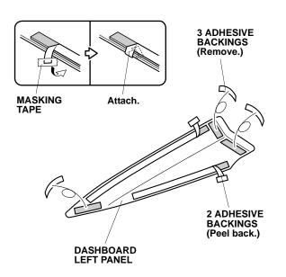
7. Align the dashboard left panel and attach it as shown.
