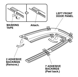
3. Align the left front door panel and attach it as shown.
