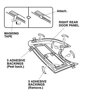
30. Align the right rear door panel and attach it as shown.
